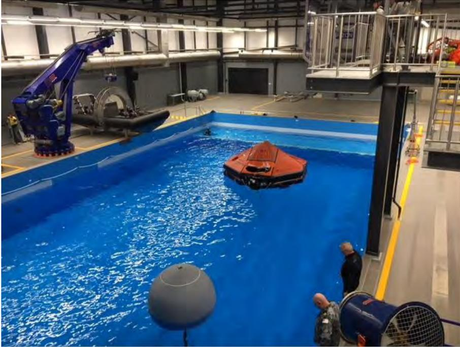
*Note the wave ball and wind fans used to simulate inclement weather.*
